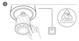
• Install Master Bulb first and then Satellite Bulb
